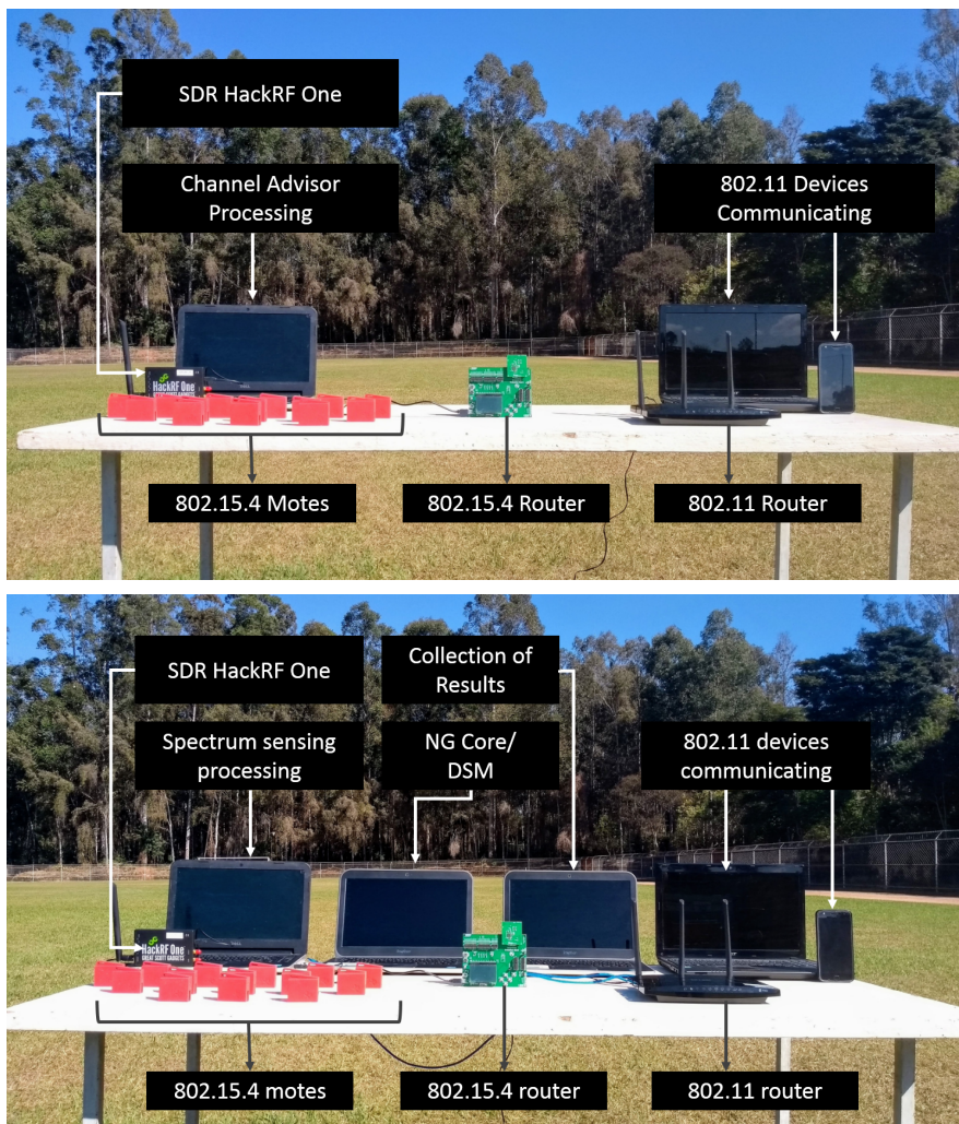
Figure 9. Experimental scenarios close to a soccer field to avoid interference to other devices outside experiment. (a) Scenario without NG; (b) Cognitive radio system scenario interoperating with NG.
