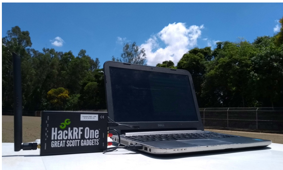
Figure 1. Hardware used to run the sensing cell module and the channel advisor (CA) firmware.
