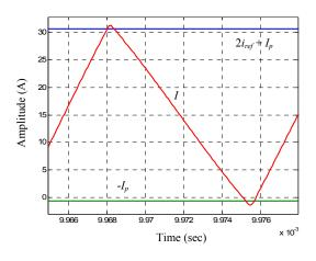
Figure 10. Inductor current for  $I_{ref} = 15 A$
