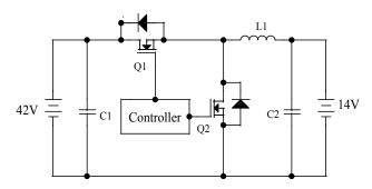
Figure 2. Basic topology of the bi-directional dc/dc converter
