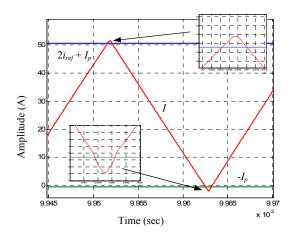
Figure 9. Inductor current for  $I_{ref} = 20 \text{ A}$
