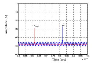
Figure 17. Output current for interleaving in boost mode
