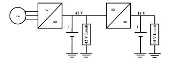
Figure 1. Block diagram of the dual voltage system
