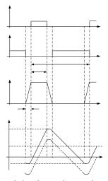
Figure 4. Gating pulses, drain voltage and current through inductance  $\mathcal{L}$ .
