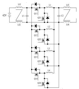
Figure 3. Interleaved bi-directional dc/dc converter.
