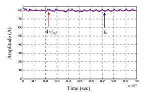
Figure 16. Output current for interleaving in buck mode
