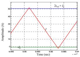
Figure 11. Inductor current for  $I_{ref} = 25 A$
