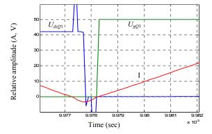
Figure 14 Zero voltage for the lower transistor  $Q_1$
