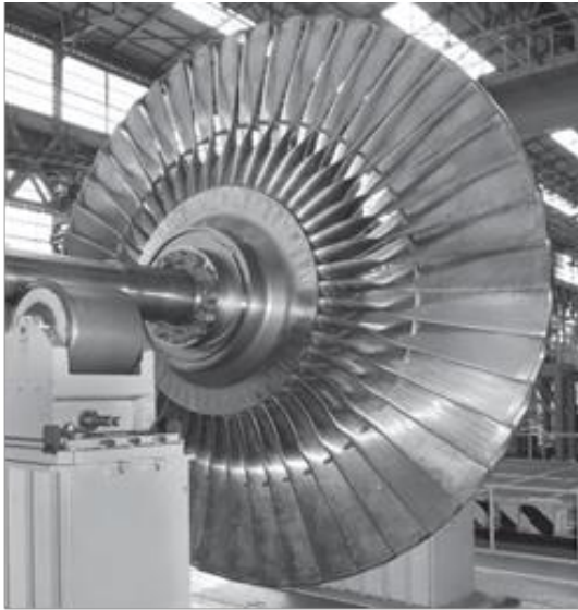
Fig. 1.4. 60-inch last-stage blades for steam turbines (Hitachi).
