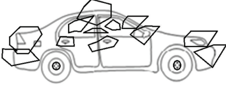
FIGURE 13: Regions containing the location of parts of interest for lateral views of vehicles, as a result of training over a representative collection of images of different types of automobiles.
