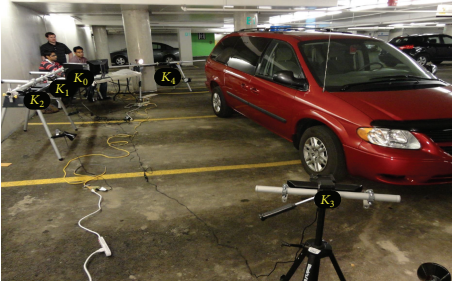
FIGURE 22: Capturing 3D data over a vehicle with the network of Kinect sensors.
