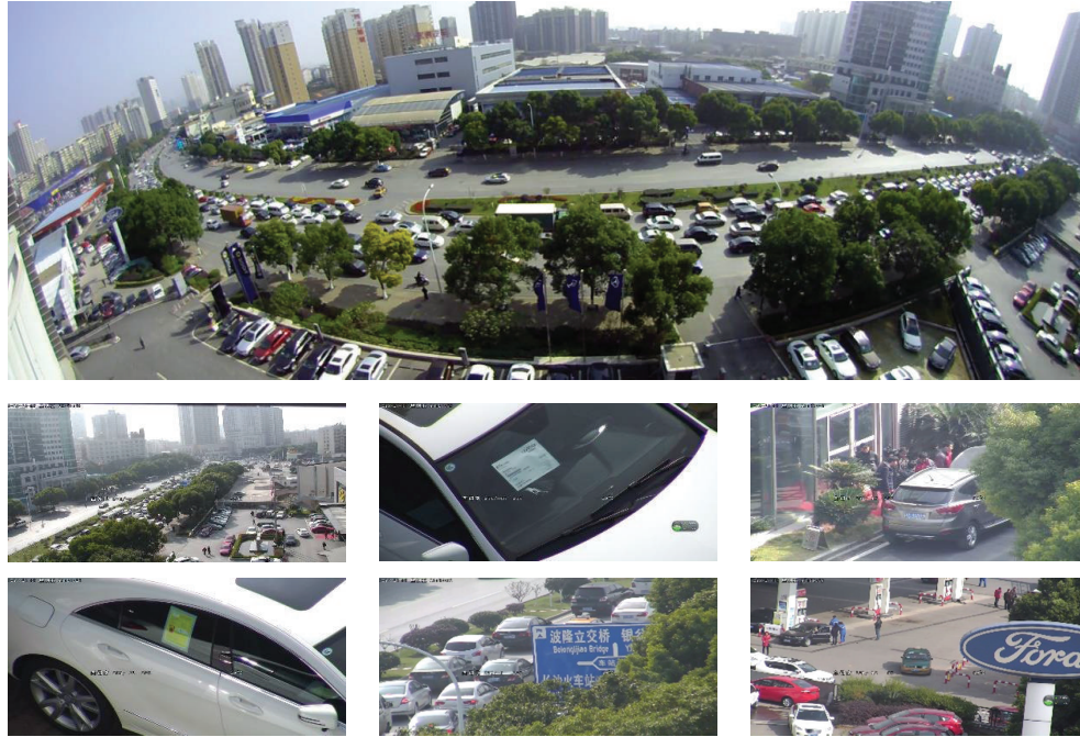
FIGURE 7: Experimental result after the calibration. Several areas are selected in the panoramic image as focus of interest, and corresponding multiscaled image is captured by PTZ dome camera.
