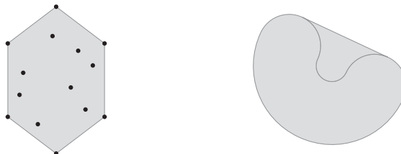
Figure 4.2: The convex hulls of two simple sets in \mathbb{R}^2 . (I) The convex hull of a set of discrete points (shown as dots) is the pentagon (shown shaded). (II) The convex hull of the kidney shaped set in Figure 4.1 is the shaded set.
