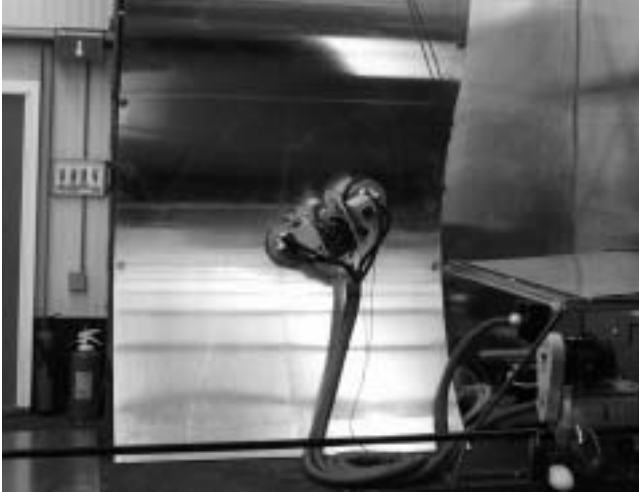
Fig. 1. The robot climbing on a curved test rig.
