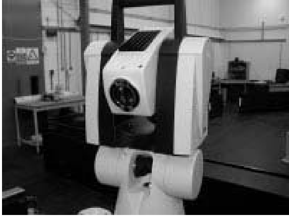
Fig. 3. A Lieca LTD-800 laser tracker.
