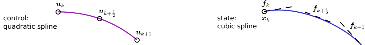
FIG. 6. Illustration of the quadratic and cubic spline segments that are used to approximate the control and state trajectories for Hermite-Simpson collocation.
