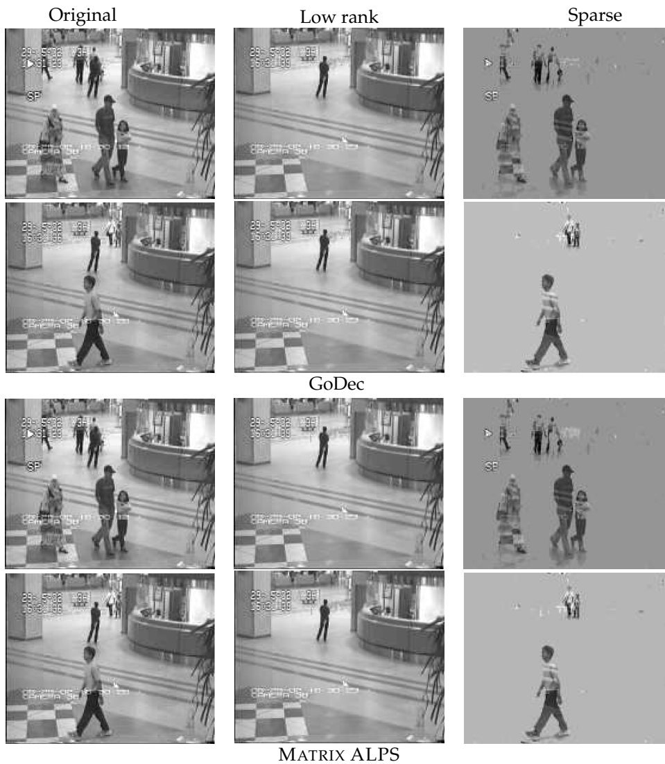
Figure 4.16: Background subtraction in video sequence. Median execution times over 10 Monte-Carlo iterations. GoDec: 34.8 sec—MATRIX ALPS: 15.8 sec.
