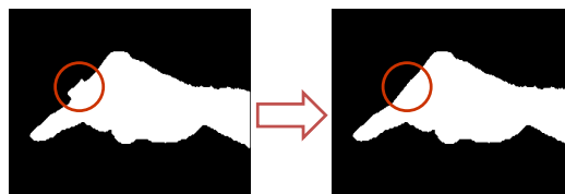
Figure 8. The elimination of noisy signals with the algorithm: S = (B \odot S) \oplus S
