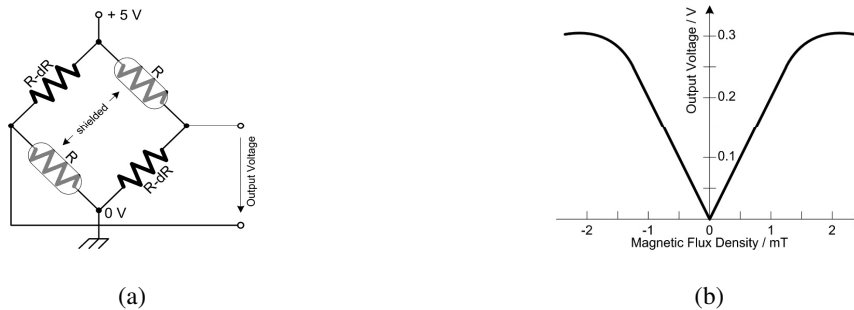
Fig. 1 (a) GMR bridge sensor AA002-02; (b) Output characteristic for a supply voltage of 5 V.
