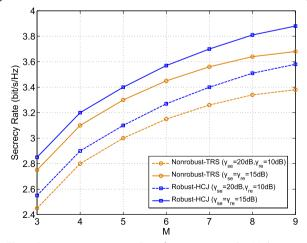
**Fig. 6** Secrecy rate versus number of cooperative nodes M, the transmit SNR is fixed as  $\gamma_{sr} = \gamma_{rd} = 40$  dB and the channel error parameter is set g = 0.3
