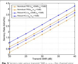
**Fig. 3** Secrecy rate versus transmit SNR  $\gamma_{sr}=\gamma_{rdr}$ , the channel error parameter is set g=0.3
