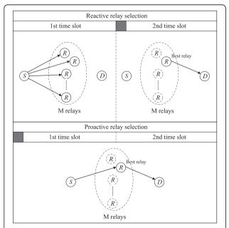
**Fig. 2** Relay selection strategy: opportunistic relay selection can be performed proactively before the source transmission or reactively after the source transmission [21]. The grade band indicates when relay selection occurs
