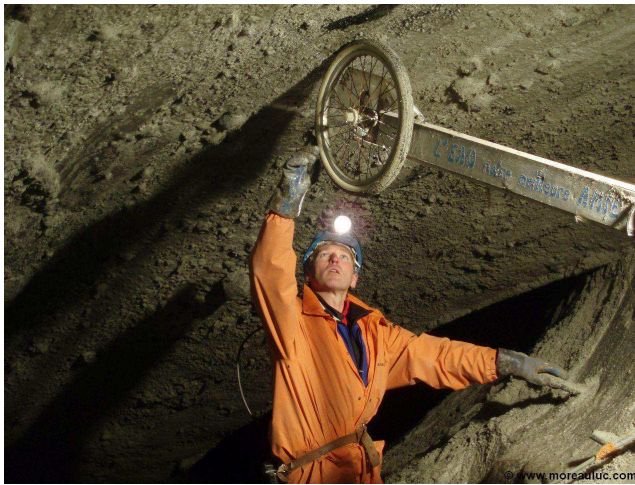
(a) Odometer in a cavity under the Argentière glacier.
