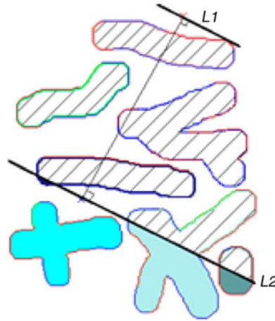
Fig. 7. Approach used to select a barrier between the start point and target: both L1 and L2 are perpendicular to the connection between the last point of current path and target. All barriers contained in the shadowed area are the selected barriers. All sub-edges that belong to the selected barrier are selected sub-edges for jump.
