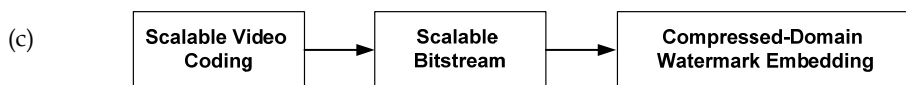
Fig. 3. Three different watermarking embedding schemes by using spatial Scalable Video Coding (Meerwald, P. & Uhl, A., 2010a): a) Watermark embedding prior to the video encoding; b) Integrated watermark embedding and coding; and c) Compressed-domain embedding after encoding.
