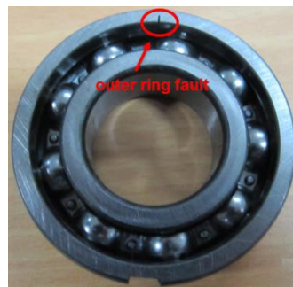
Figure 13. Bearing outer ring fault.
