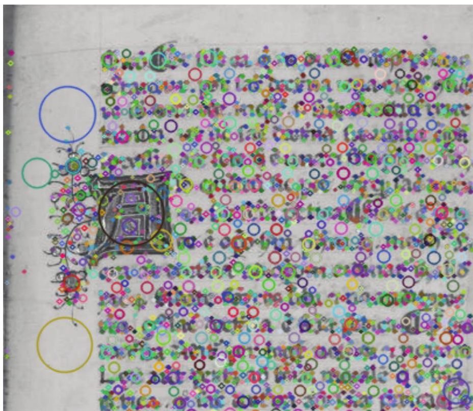
Fig. 3. Visualization of SIFT keypoints (Toulouse, Bibliothèque municipale, MS 214). The (randomly colored) circles visualize the local scope of the features. Note also that SIFT keypoints that lie between two lines may contain information about, for example, the typical line height and ascenders or descenders.
