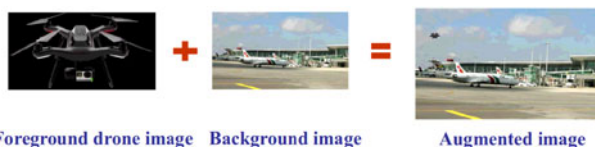
Fig. 3. Illustration of the data augmentation idea, where augmented training images can be generated by merging foreground drone images and background images.
