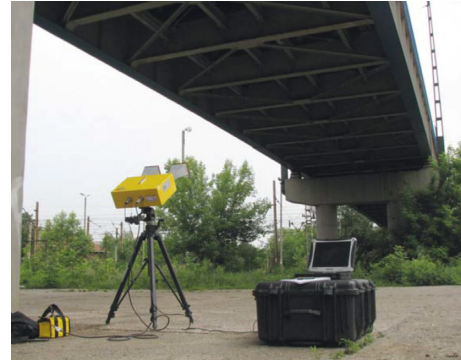
FIGURE 9: IBIS-S radar unit under the tested bridge span.
