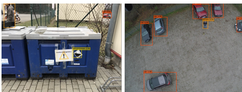
Figure 7. Object detection example: GHS (Globally Harmonized System of Classification, Labelling and Packaging of Chemicals) pictogram, person and vehicle. Number corresponds to confidence in [0,1] .
