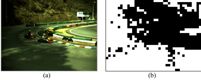
Figure 3. (a) Original frame of Race1 sequence (b) Low textural region in white and high textural region in black
