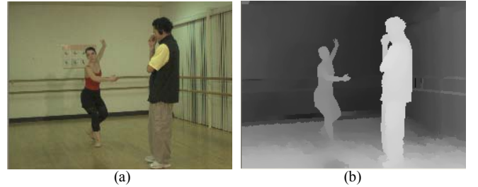
Figure 2. Pixel map and depth map of the first frame on view 1 for “Ballet” sequence. (a) Pixel map. (b) Depth map.
