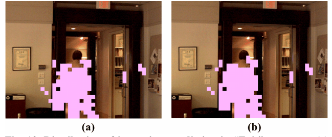
Fig. 10. Distribution of inter-view prediction in “Exit” sequence. (a) After estimation of Inter16×16 mode. (b) After estimation of all Inter modes.
