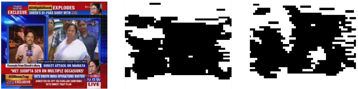
Figure 7.1: Output of the change detection (a) Rectangular bands detected from Hough Lines, (b) Output of the pixels based change detection with N = 50 , (c) Output of the histogram based change detection with N = 50 .
