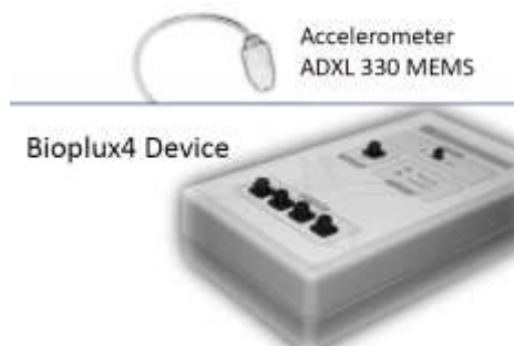
Figure 4.1 – Bioplux4 Device and Accelerometer ADXL 330 MEMS
