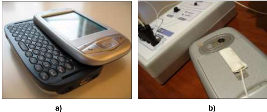
Figure 4.12 – a) HTC Wizard PDA; b) HTC Wizard with ADXL 330 accelerometer
