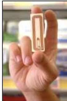
Figure 2.1 – One kind of RFID tag
