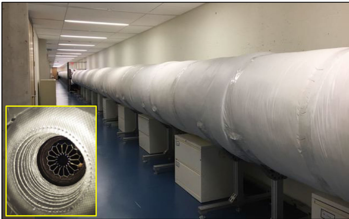
Figure 6.4-1. S5’s starshade model validation testbed at Princeton. Model starshade shown in inset.
