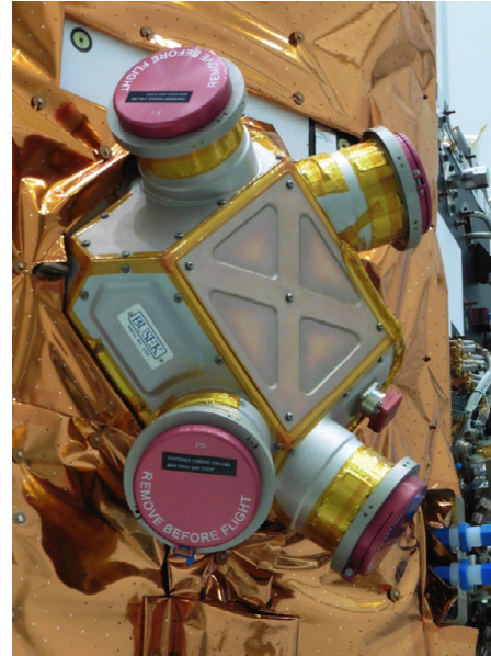
Figure 6.4-4. A single cluster of four Busek Co. colloidal microthrusters integrated on the LISA-Pathfinder Spacecraft just prior to launch. Image courtesy ESA / Airbus.
