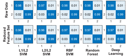
Fig. 11. Normalized confusion matrices for binary classification task. Vehicle classes: 1: Car-like, 2: Truck-like.
