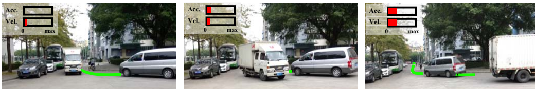
Fig. 1: A typical scenario we explore in this paper. The gray van tries to turn right. Seeing the white truck, it decelerates and waits at the junction. After the white truck passes by, it accelerates and follows the planned path. The green curve shows the planned path and the upper left insets show the velocity and acceleration of the gray van at different moments.
