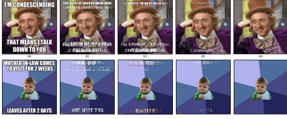
Figure 2: Sample recovery of the template images “Willy Wonka” and “Success Kid” from the target set examples. We show the obtained template at (a) 0 iterations, (b) 10 iterations, (c) 20 iterations, (d) 50 iterations and (e) 100 iterations.
