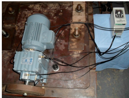
Figure 1. An experimental rig of simulating gear faults.
