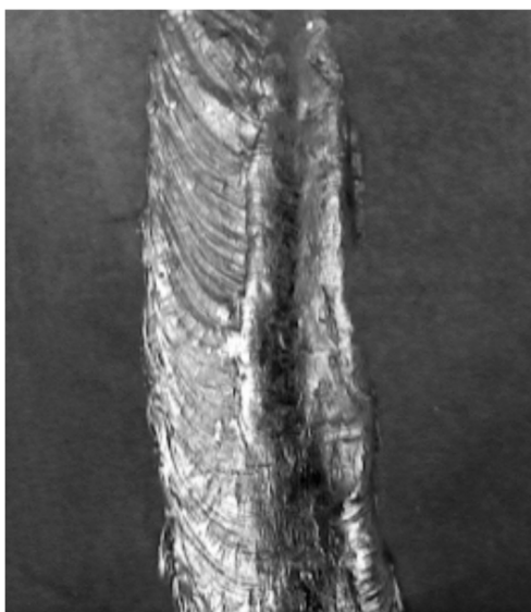
Figure 1. Laboratory sample of an OK weld.
