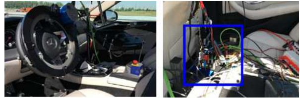
Fig. 12 Examples of instrumented car with equipment: (a) Control equipment (b) Measurement equipment.
