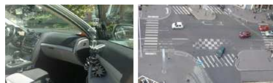
Fig. 5 Two types of naturalistic observations were carried out: (a) Video data from in-vehicle camera (b) View from infrastructure-mounted cameras.
