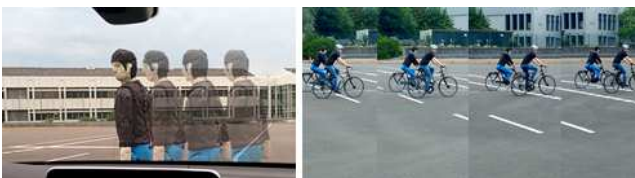
Fig. 11 Examples of advanced dummy features: (a) Pedestrian dummy full stop and rotate head towards approaching car, (b) Pedaling cyclist dummy with rotating wheels.
