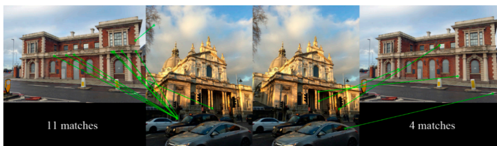
Figure 7. Different matching results of two matching directions.
