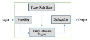
Fig. 1. The structure of fuzzy logic system
