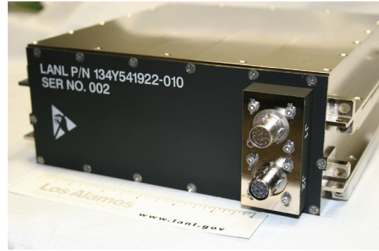
FIGURE 11: Completed, sealed T-SDR system with satellite interfaces.
