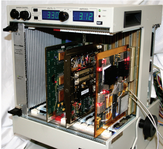
FIGURE 10: T-SDR modules loaded in a compact-PCI test chassis. The use of commodity compact-PCI chassis allow for cheap and efficient development cycles. Shown right to left are RTSP, DCR, and SVIM in COTS cPCI test chassis.
