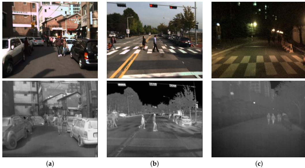
Figure 1. Examples of various light conditions and their influence on the visibility of people in visible light (first row)/thermal (second row) images: (a) Warm day with good visibility in bright regions and low contrast in the shadow in RGB; low contrast in thermal range. (b) Good pedestrian visibility in both visible light and thermal images. (c) Night scene with low visibility in RGB and pedestrians visible in thermal.
