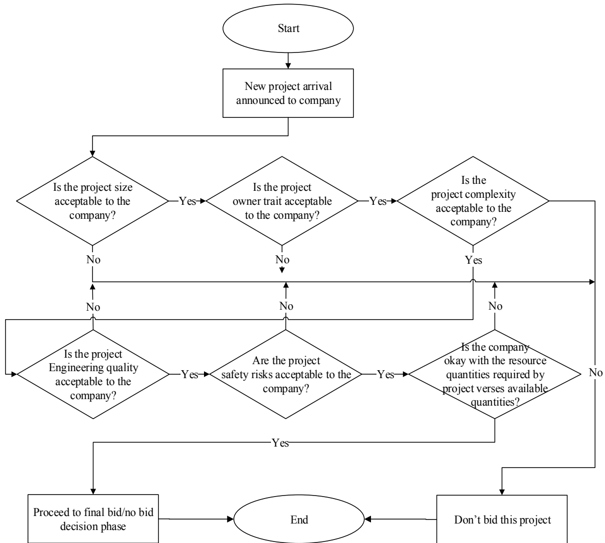
Figure 5.26: Process Flow Logic used By Company Agents to make their Initial Bid/No Bid Decision
