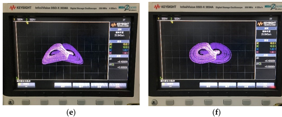
Figure 16. Experimental results obtained by Digital Signal Processing (DSP) technology. (a) Chaotic pseudo-noise (PN) sequence extracted from the variable x , (b) chaotic attractor on the x - y plane, (c) chaotic attractor on the y - z plane, (d) chaotic attractors on the x - z plane, (e) coexisting attractors on the y - z plane, (f) coexisting attractors on the x - z plane.
