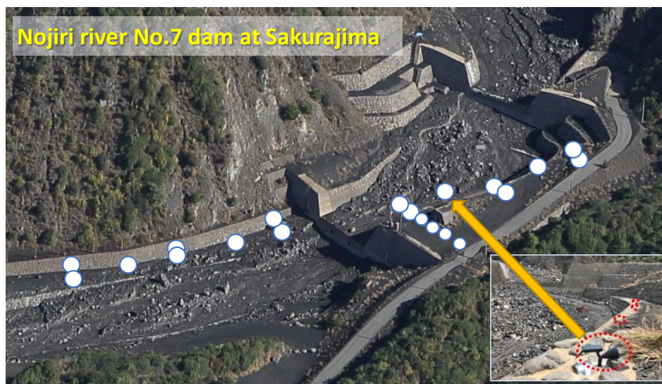
Figure 5. The deployment map of monitoring sensors, in which accelerometer sensors are marked with white circles.
