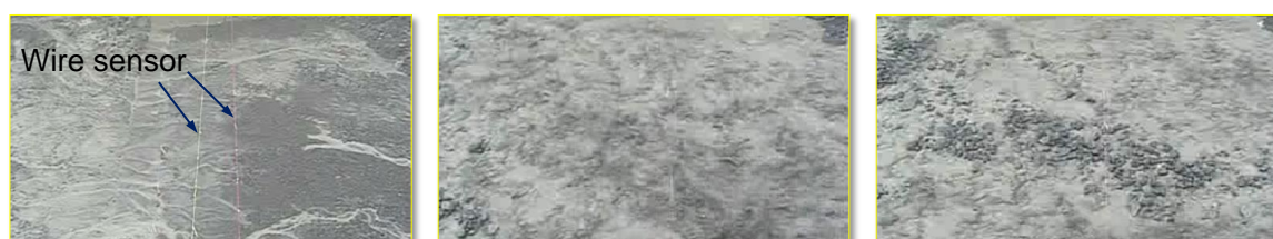
Figure 9. Snapshots of wire sensor utility. The conditions of before/during/after debris flow strikes are shown from left to right, respectively.
