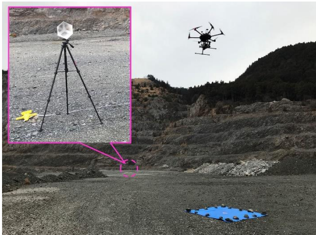
Figure 9. Data acquisition test targeting a corner reflector
