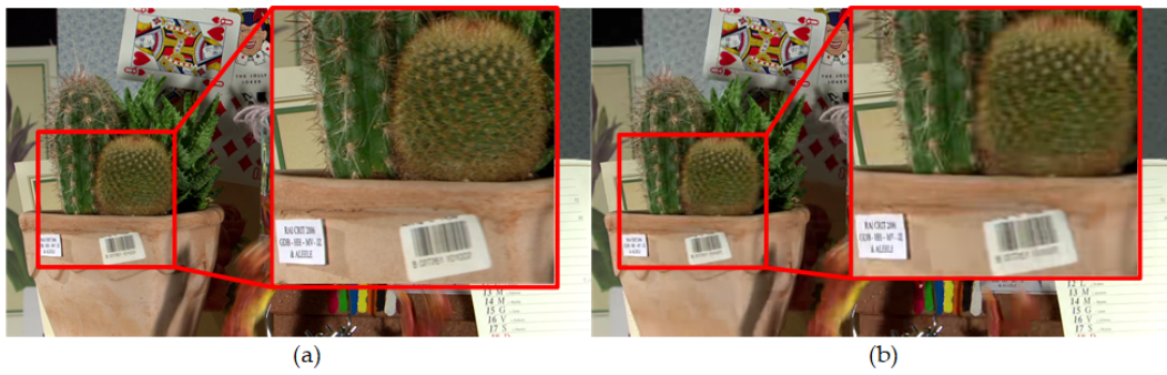
Figure 13. The 34th encoded frame of the Cactus video sequence with QP = 19 and QP = 40 under the RA mian10 configuration of HM 16.9. (a) The subjective and objective quality (PSNR) of the encoded frame is 40.10 dB with QP = 19; (b) the PSNR of encoded frame is 31.30dB with QP = 40.
