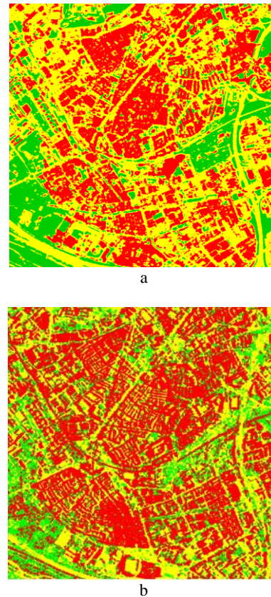
Figure 3. SVM classification result on a) SPOT, b) SAR
