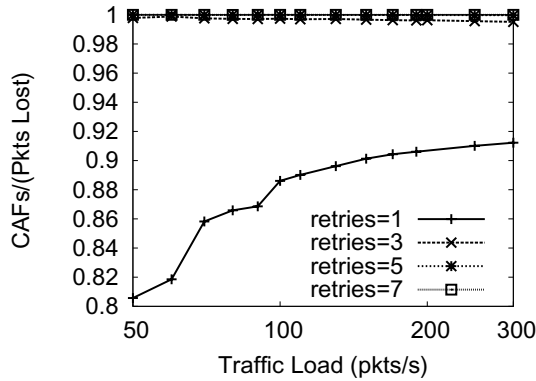
Fig. 9. Ratio of channel access failures to total number of lost packets in simulations with different macMaxFrameRetries values in the absence of hidden nodes.
