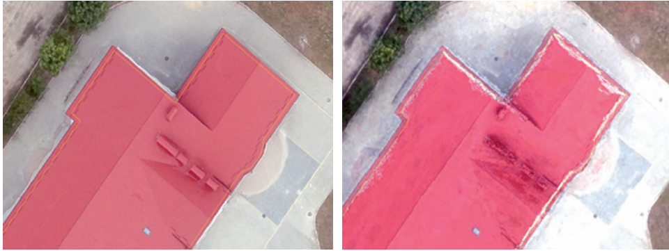
Fig. 2. Fragments of a building's image on a traditional orthophotomap (left) and on the orthophotomap designed using the proposed method (right)
