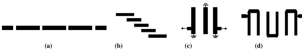
Figure 2. 11 Example of bandpass filter design structures a) end-coupled, b) edge -coupled, c) interdigital, and d) hairpin lines
