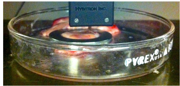
Fig. 18 Experimental nanoindentation setup. A 5 mm-thick coronal slice of freshly harvested brain tissue is placed in a 100mm-diameter petri dish and mounted underneath the force transducer of the TriboIndenter™. A 12 mm-diameter washer marks the indentation region and stabilizes the sample. A circular flat punch of 1.5 mm diameter ensures a homogenized specimen response. Reprinted with permission from [20]
