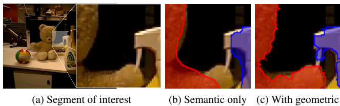
Figure 4: Comparison of boundaries produced by semantic labelling only and by merged semantic and geometric labelling. While the semantic segmentation is smooth, it lacks important details.
