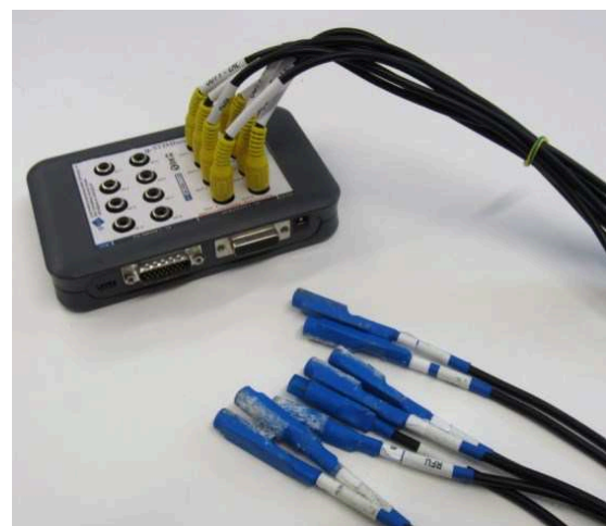
Figure 1: Eight g.VIBROstim stimulators plugged into the g.STIMbox that drives them
