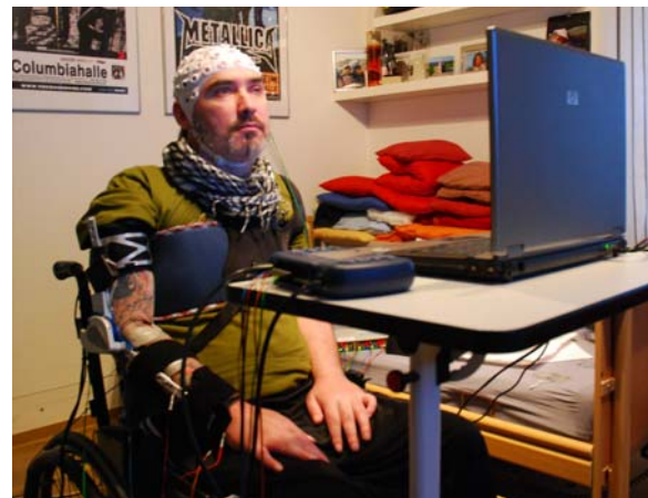
Figure 1: End user of the modular upper extremity neuroprosthesis during a BCI classifier setup session
