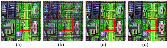
Fig. 12. Denoising results of the Washington DC Mall image in Case 3: (a) original false-color image (R: 180, G: 61, and B: 9); (b) noisy band; (c) LRMR; and (d) NAILRMR.
