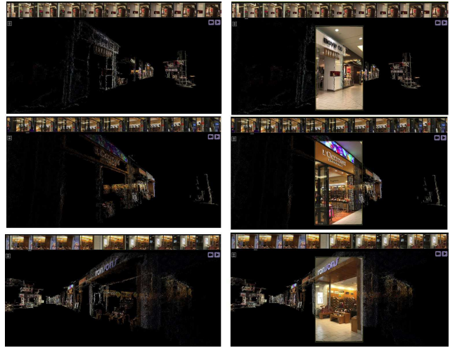
Figure 6: Virtual navigation. Left: virtual navigation; right: overlaying of video frames on top of the 3D visual model. User can explore by themselves in 3D space.
