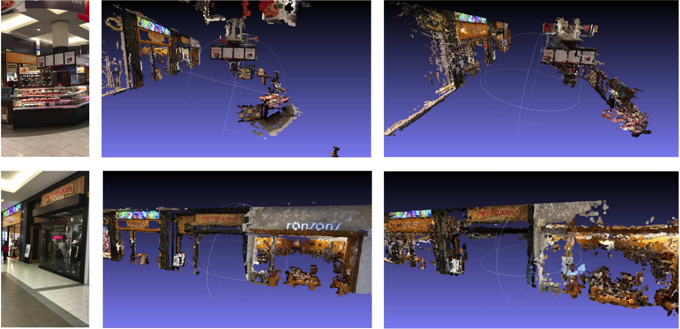
Figure 9: Comparison of 3D visual model details. Left: original video frame; Middle: OpenMVG results; Right: vsfm results.
